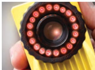
Integrated ring lights provide basic lighting for In-Sight vision sensors.
